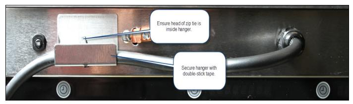
The cord hanger is attached to the cabinet with double-stick tape opposite the rear-mounted strain relief.
